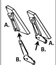
When assembling back to arms, place Bracket B Into Sleeve A and press top of back down firmly to lock the retaining clip into place. Listen for the clip to pop into place – and your KD back is securely in place!
